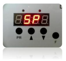
Activate the PR key again and the temperature to be set to work appears flashing on the screen.
