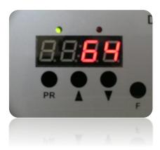
Activate the ▲ key to increase the cooling plate temperature value.
