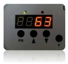
Click again on [PR] button and hold it for 5 seconds to confirm the set value. Then the SP message and then the internal current temperature from tank appear on the screen.
